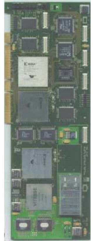
A Dag 4.1 card - designed for passive network monitoring at 2.5 Gb/sec (OC48c network links).
